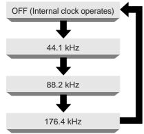
Press the EXT. CLOCK button to match the frequency with the clock frequency set in the master clock generator, and when the LOCK indicator switches on, the settings are complete.
