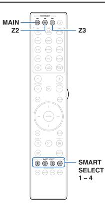
Settings such as the input source, volume level and sound mode can be registered to the SMART SELECT 1 - 4 buttons.
