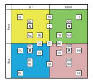
For example, if "Subwoofers" = 2 spkrs and Subwoofer Layout = Left/Right, Subwoofer Left (Subwoofer 1) plays the bass of the speakers in the Left area which includes FL/SL and Subwoofer Right (Subwoofer 2) plays the bass of the speakers in the Right area which includes FR/SR.
