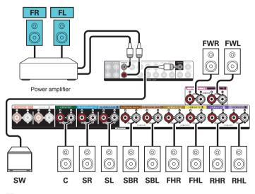
When connecting 13.1 channel speakers, an external amplifier needs to be connected to the Front channel or the Front Wide channel at minimum. Set "Connection" to "Pre-out Only" for your preferred channel. (127) p. 230)
