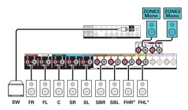
\* The height speakers, ceiling speakers and Dolby Atmos Enabled speakers can be connected to the HEIGHT1 speaker terminals. Set the speaker to be connected from "Speaker Layout" in the menu. ((27 p. 230))
