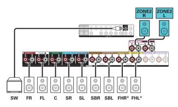
\* The height speakers, ceiling speakers and Dolby Atmos Enabled speakers can be connected to the HEIGHT1 speaker terminals. Set the speaker to be connected from "Speaker Layout" in the menu. (137 p. 230)
