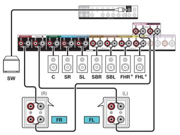
\* The height speakers, ceiling speakers and Dolby Atmos Enabled speakers can be connected to the HEIGHT1 speaker terminals. Set the speaker to be connected from "Speaker Layout" in the menu. (127 p. 230)
