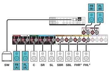
\* The height speakers, ceiling speakers and Dolby Atmos Enabled speakers can be connected to the HEIGHT1 speaker terminals. Set the speaker to be connected from "Speaker Layout" in the menu. ((27 p. 230)
